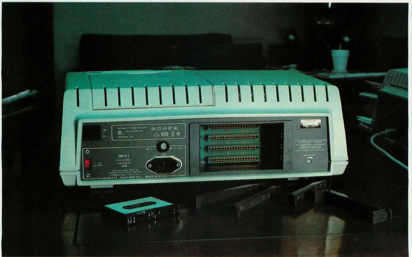
Photo 4: Rear view, showing the four I/O ports and their removable covers.
